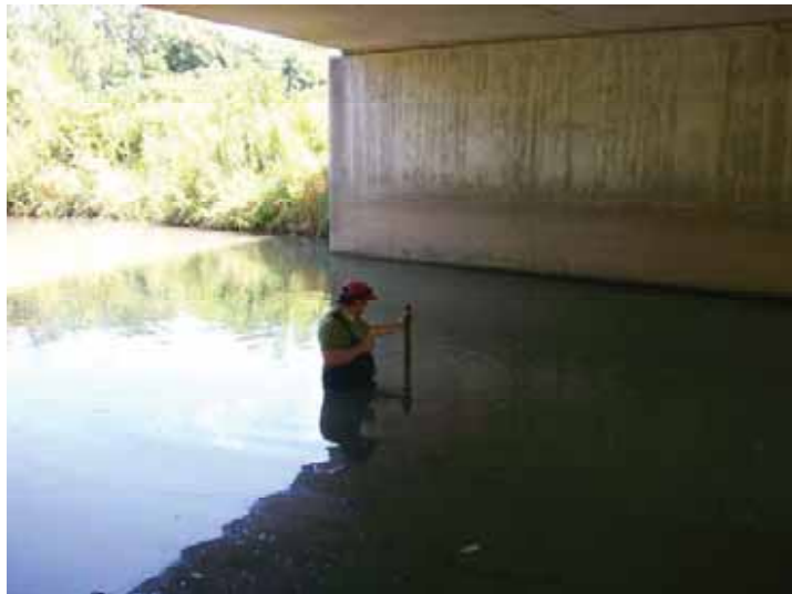
Photo 151: View of Mud Creek facing northeast (August 14, 2014). The OHWM is 27 feet wide and 54 inches deep.
